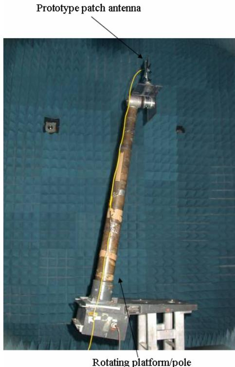
Figure 5. Radiation pattern measurement setup in the anechoic chamber.
