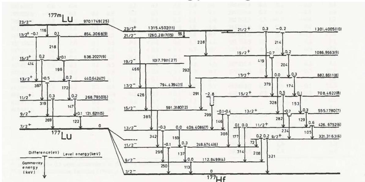
Figure 4. Decay Scheme of  $^{177m}\text{Lu}$ . Shown are the level energies, spins, and level differences that created the released gamma energies.
