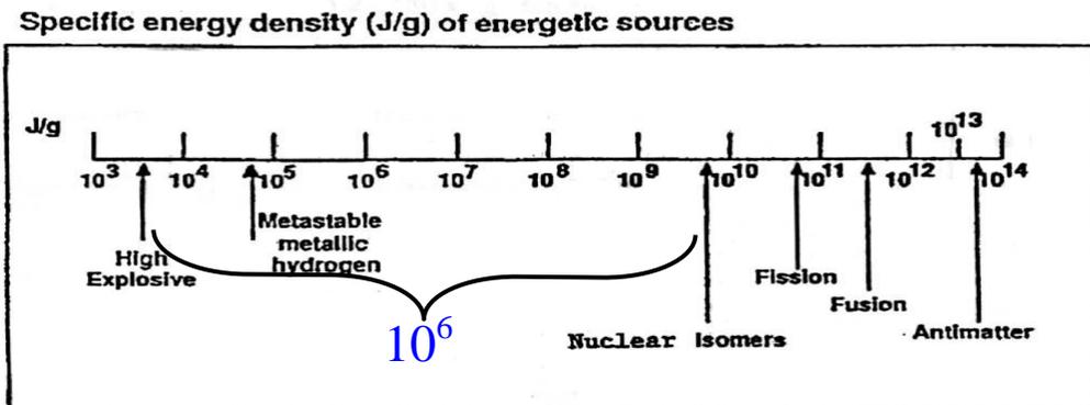
Figure 5. The energy density of nuclear sources exceeds that of chemical energy densities by more than six orders of magnitude.
