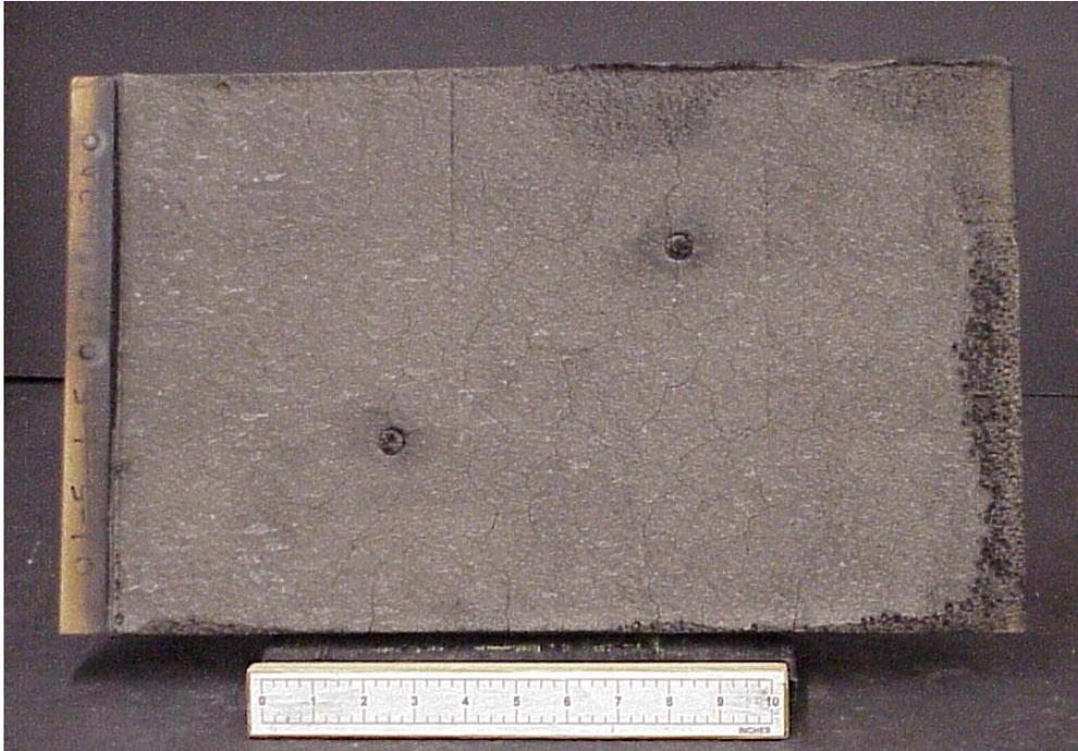
**Figure 3-3. Post Test Photo of Intumescent 1 Panel 1**
