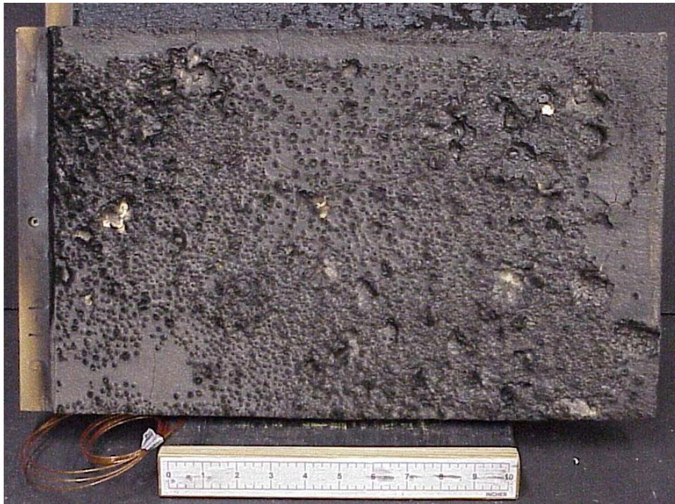
**Figure 3-4. Post Test Photo of Intumescent 1 Panel 2**
