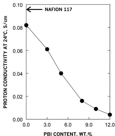
**Figure 8** – The effect of PBI content on the measured proton conductivity (at 24°C) of water-equilibrated SPOP-PBI blended membranes. All membranes prepared with 1.4 IEC SPOP.
