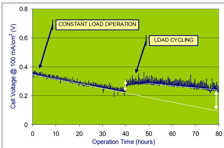
**Figure 16** – Voltage vs. time plot for long-term MEA testing with an SPOP-PBI membrane. 1.0 M methanol 60°C, 100 mA/cm<sup>2</sup> load.
