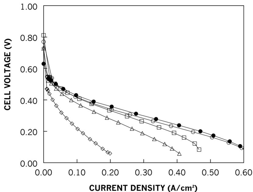
**Figure 12** – Electrochemical performance of SPOP-PBI blended membranes in a direct methanol fuel cell (60°C, 1.0 M methanol, air at ambient pressure).
