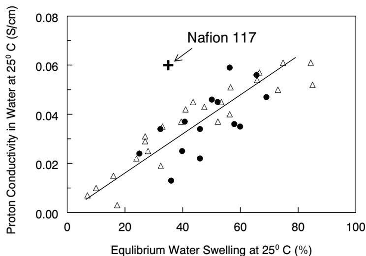
**Figure 4** - Correlation of membrane proton conductivity vs. equilibrium membrane water swelling for SMPOP/Flex membranes. Conductivity measured by AC impedance for membranes immersed in water. Open triangles are UV-crosslinked membranes; solid circles are electron-beam-crosslinked films.
