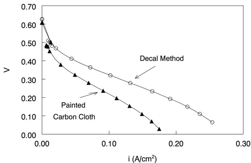
**Figure 7** - Comparison of MEA Fabrication Methods. Membrane: Nafion 117, Cell Temp. = 60°C; 1 M methanol; Air at 70°C, 600 SCCM and 30 psi; Anode = 4 mg/cm<sup>2</sup> Pt-Ru w/10% SMPOP binder; Cathode = 2 mg/cm<sup>2</sup> Pt-black w/8% PTFE binder + 2 mg/cm<sup>2</sup> Pt-black w/10% SMPOP Binder; electrode geometric area = 5 cm<sup>2</sup>.
