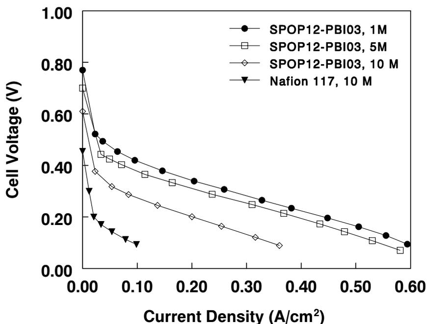
**Figure 13** – Electrochemical performance of a SPOP12-PBI03 MEA in a direct methanol fuel cell at different methanol feed concentrations (60°C and air at ambient pressure and 500 sccm). SPOP-PBI membrane thickness was 82  $\mu\text{m}$ .
