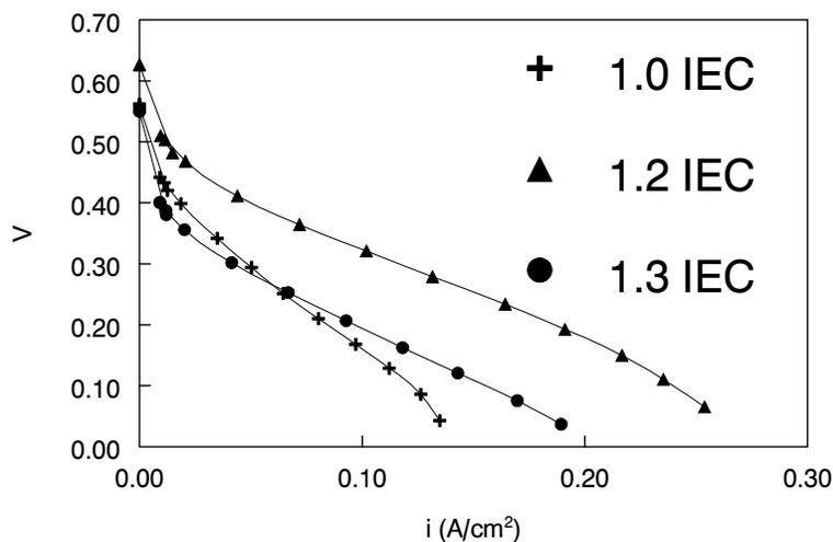
**Figure 6** - The effect of SMPOP binder IEC on DMFC performance. Membrane: Nafion 117, Cell Temp. = 60°C; 1 M methanol; Air at 70°C, 600 SCCM and 30 psi; Anode = 4 mg/cm<sup>2</sup> Pt-Ru w/10% SMPOP binder; Cathode = 2 mg/cm<sup>2</sup> Pt-black w/8% PTFE binder + 2 mg/cm<sup>2</sup> Pt-black w/10% SMPOP Binder; electrode geometric area = 5 cm<sup>2</sup>.
