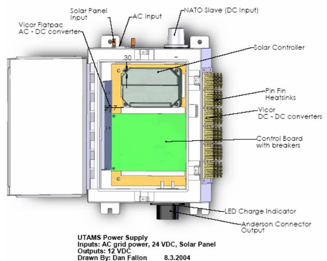
Fig. 2. UTAMS power supply box, interior view.
