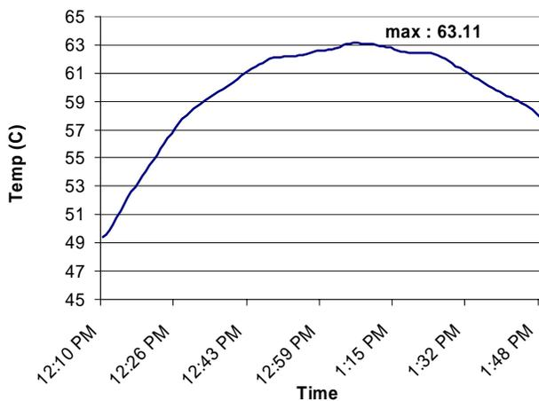
Fig. 3. Temperature rise of enclosure at near full power in full sun, 90F ambient.
