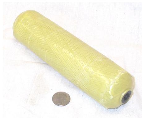
**Fig. 10.** Kevlar/epoxy tank surrounding monolith
