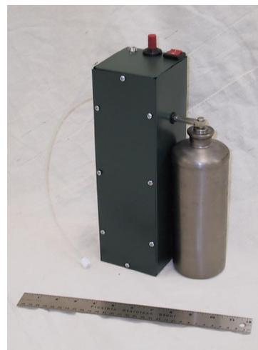
**Fig. 3.** Ammonia-based hydrogen generator
