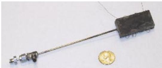
**Fig. 2.** MesoChannel™ ammonia-decomposition reactor
