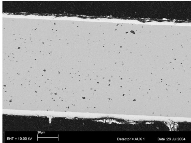
*Figure 1 Electron micrograph of section through the 100  $\mu\text{m}$  thick YSZ sheet. The dense white layers on the top and bottom are of barium zirconate, the desired buffer layer. That the surface film is  $\text{BaZrO}_3$  was confirmed using electron-dispersive x-ray energy analysis and x-ray diffraction. (The dark spots within the YSZ substrate were analyzed to be  $\text{Al}_2\text{O}_3$  – but we have no idea why these are present in the material.)*
