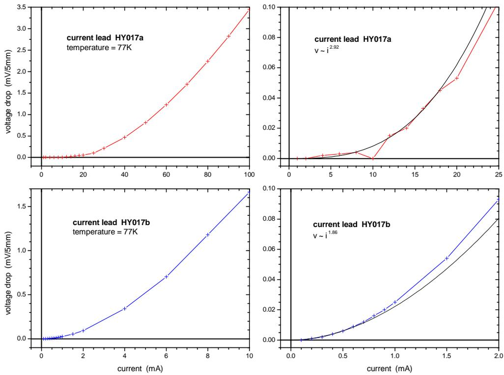
Figure 3: *V-I data for two  $YBa_2Cu_3O_7$  strips laid on  $BaZrO_3$  buffered YSZ substrates.*
