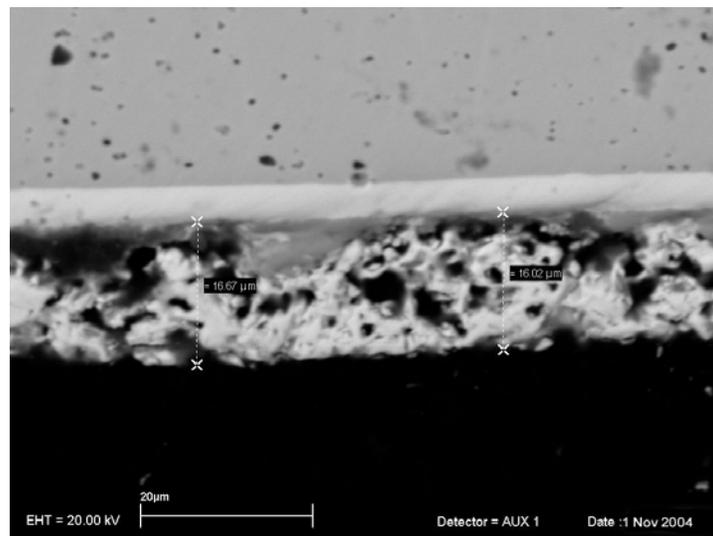
Figure 4: *Cross-section of current lead. The YSZ substrate lies at the top of the micrograph – and contains particulate  $Al_2O_3$  (the dark spots). A dense layer of  $BaZrO_3$ ,  $\sim 4 \mu m$  thick has been formed at the substrate surface; and a porous layer of  $YBa_2Cu_3O_7$ ,  $16 \mu m$  thick, has been sintered on the surface of the  $BaZrO_3$ .*
