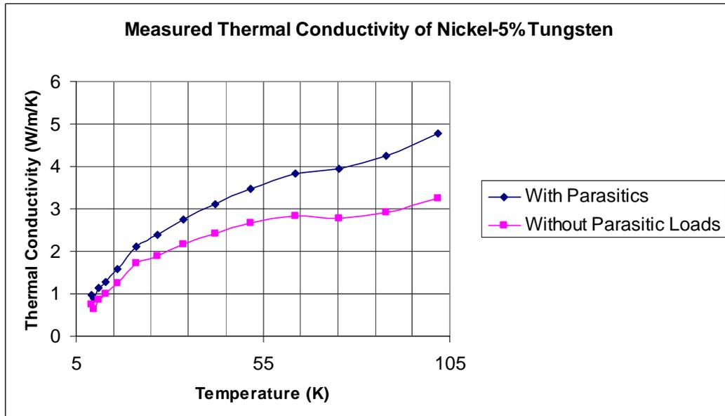
Figure 10: Measured thermal conductivity of Nickel-5% Tungsten substrate.
