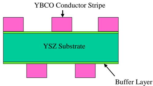
Fig. 1 Showing a cell of 5 conductor stripes in a 2-sided configuration. Each stripe is designed to operate up to a current of 100mA ( $I_c = 200\text{mA}$ ). The expected route mean square operating current per stripe is 35mA.
