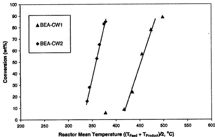
Fig. 5. Effect of reactor temperature on cracking conversion in coated wall reactors at LHSV = 100 h<sup>-1</sup>.
