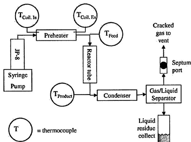
Fig. 2. JP-8 catalytic cracking experimental setup.
