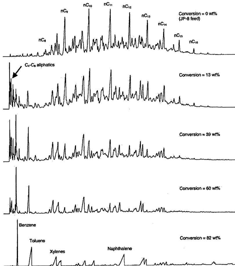
Fig. 8. GC-FID chromatograms of liquid residue from JP-8 catalytic cracking on Mn/ $\gamma$ -alumina catalyst.
