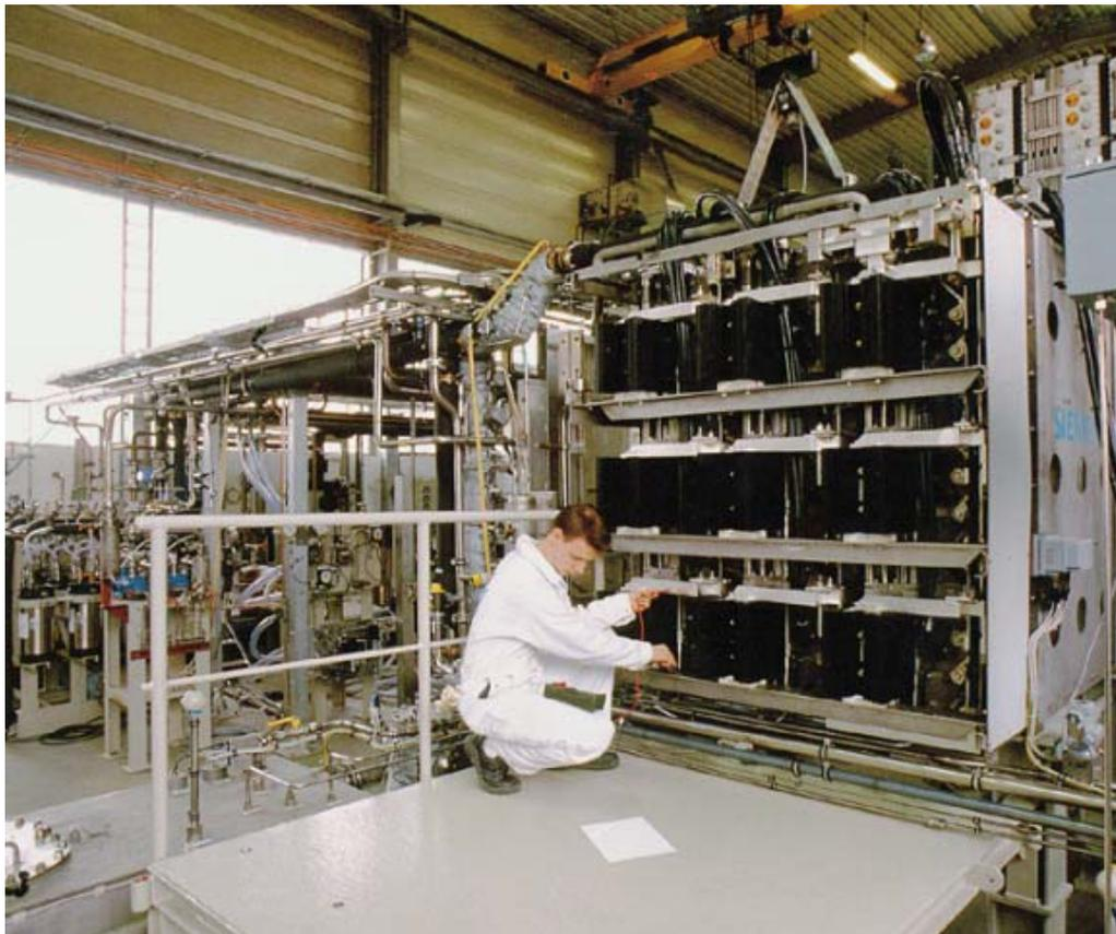
Figure 4: A Siemens 300 kW PEMFC Stack Assembly as used on the German 212 AIP Submarine (Copyright Jane's Information Group; Source: HDW).
