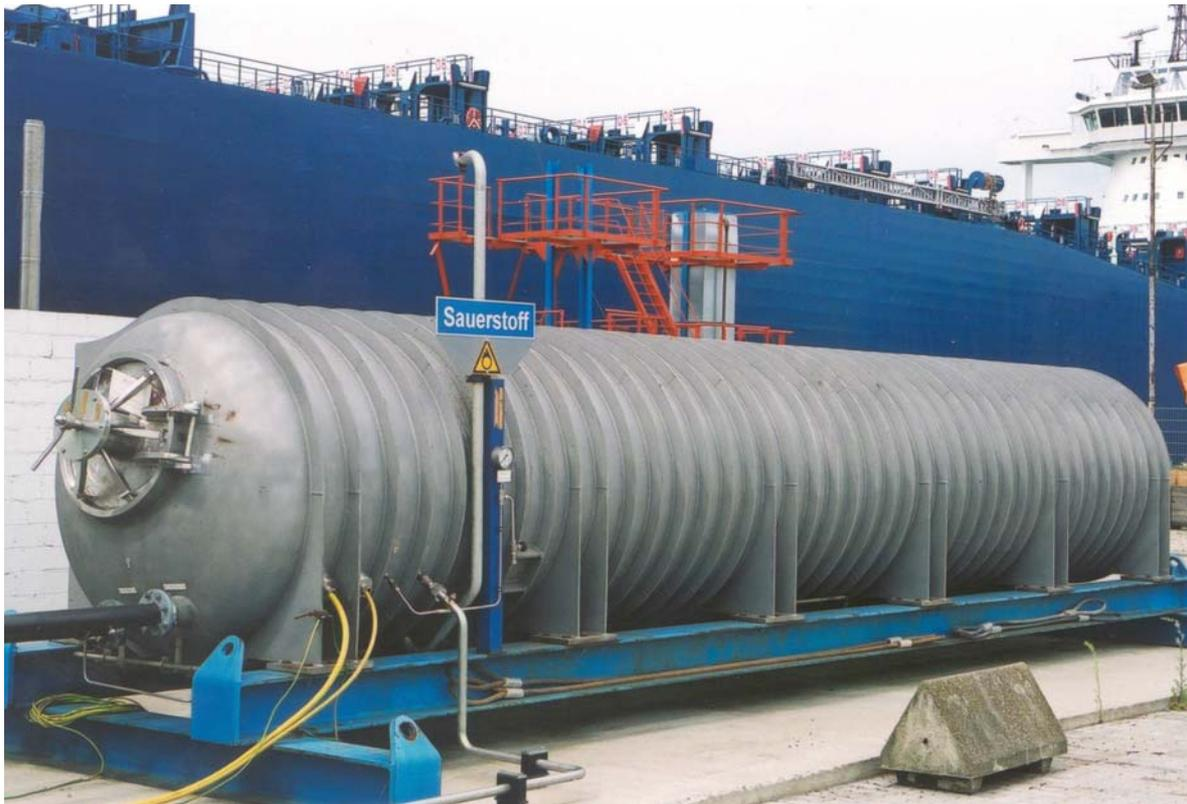
Figure 7: A LOX Tank on the German 212 AIP Submarine (Source: HDW).
