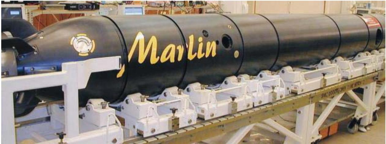
**Figure 10: The 21-inch, Tube Launched, Mine Reconnaissance Vessel Marlin.**
