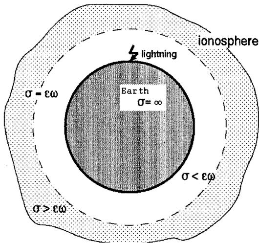
Fig. 1. Configuration of the Earth-ionosphere cavity.
