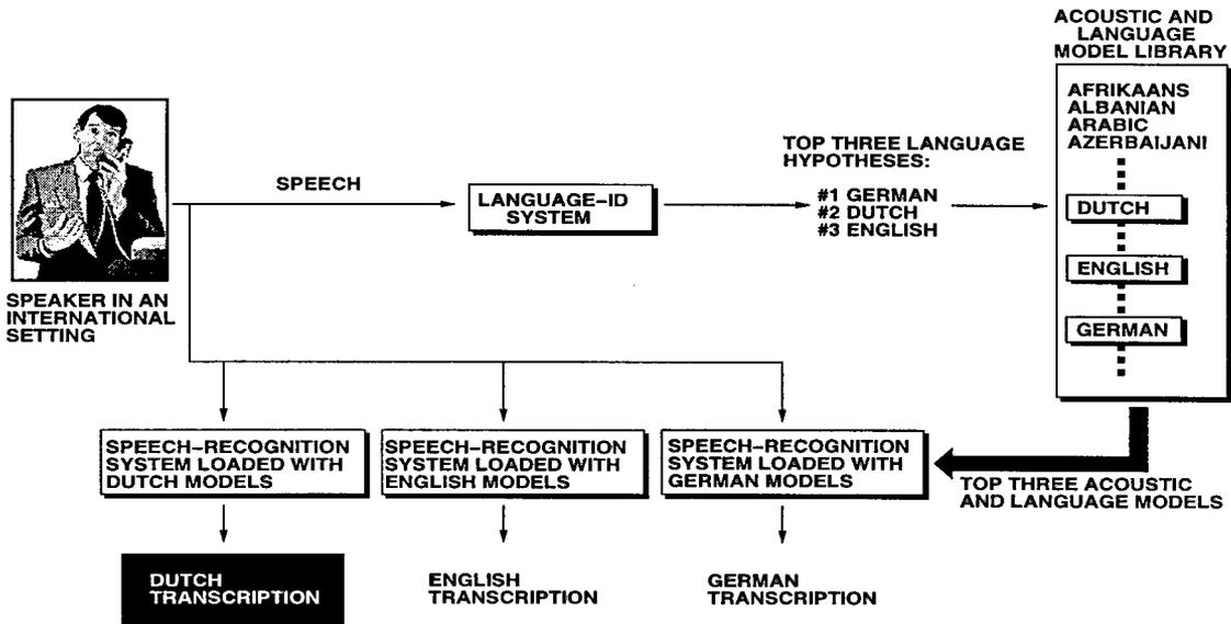
Figure 1: A language-identification (LID) system as a front end to a set of real-time speech recognizers. The LID system outputs its three best guesses of the language of the spoken message (in this case, German, Dutch, and English). Speech-recognizers are loaded with models for these three languages and make the final LID decision (in this case, Dutch) after decoding the speech utterance.
