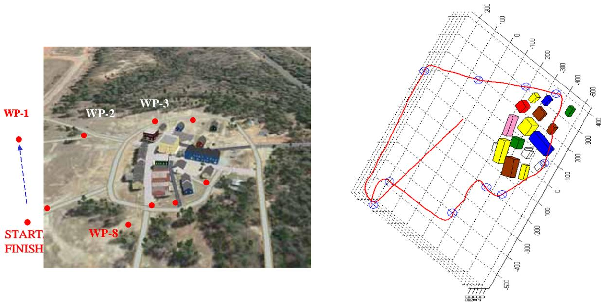
**Figure 4:** Figure at left shows an image of McKenna MOUT with mission plan – 10 waypoints superimposed on the map. The figure at the left shows a matlab regeneration of the same map with a nominal trajectory obtained after an example flight.
