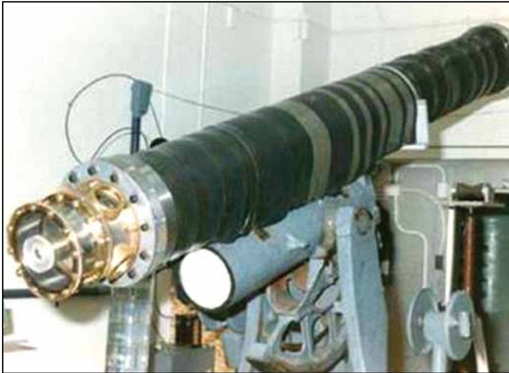
Figure 6. A Water Pulse-Forming Line and Spark-Gap Switch Test
