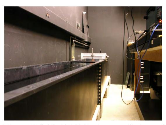
Figure 3: The test tank facility in Dr. Jaffe's lab. The tank can accommodate the range of intended imaging distances of 5 – 15 meters.
