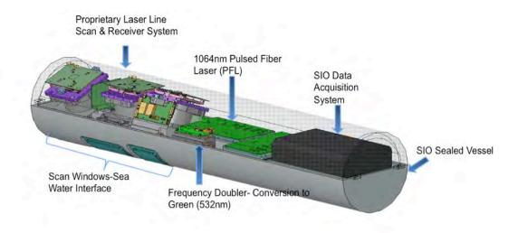
Figure 1: Prototype underwater imaging system representing the Phase II deliverable
