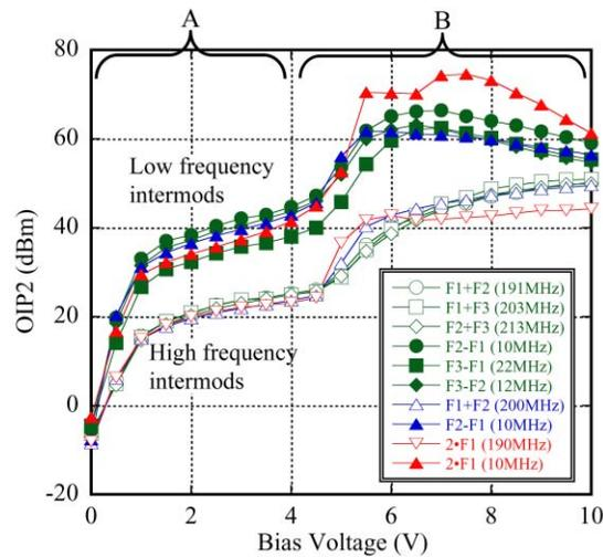
Fig. 3. OIP2 versus bias voltage for a PD3000 photodiode, using one-, two- and three-tone measurement setups. Fundamental frequency  $f = 100\text{MHz}$ , with frequency spacing  $\Delta f = 10\text{MHz}$  and total photocurrent = 10mA. One- and three-tone data are shifted according to Eq. (10) to mathematically match the two-tone data. One-tone data for 5MHz fundamental included (red solid triangles).
