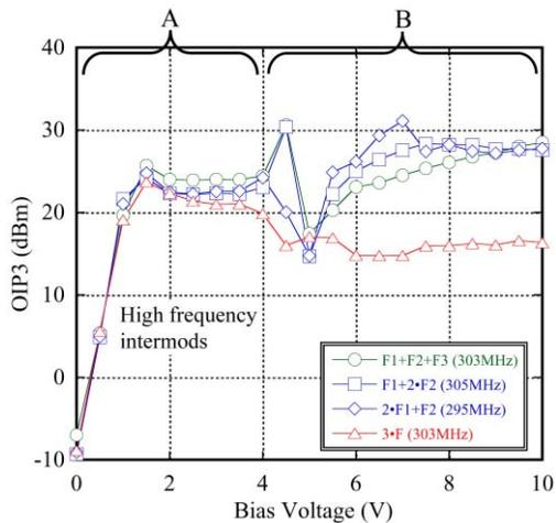
Fig. 5. OIP3 versus bias voltage for a PD3000 photodiode, using one-, two- and three-tone measurement setups. Fundamental frequency  $f = 100\text{MHz}$ , with frequency spacing  $\Delta f = 10\text{MHz}$  and total photocurrent =  $10\text{mA}$ . Only distortion near  $3 \cdot f$  is plotted. One- and three-tone data are according to Eq. (11) to mathematically match the two-tone data.
