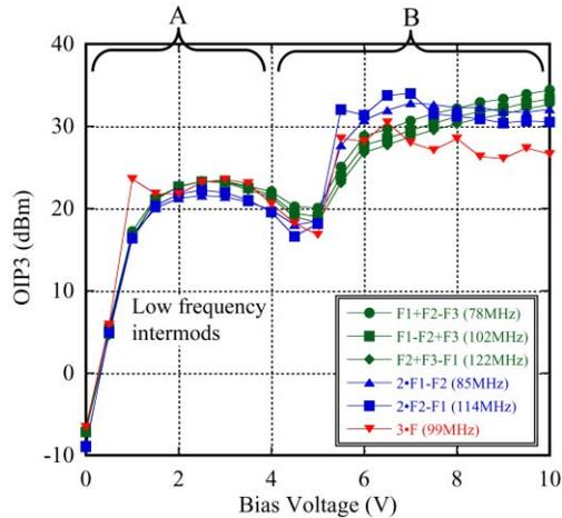
Fig. 4. OIP3 versus bias voltage for a PD3000 photodiode, using one-, two- and three-tone measurement setups. Fundamental frequency  $f = 100\text{MHz}$ , with frequency spacing  $\Delta f = 10\text{MHz}$  and total photocurrent =  $10\text{mA}$ . Only distortion near  $f$  is plotted. One- and three-tone data are according to Eq. (11) to mathematically match the two-tone data. One-tone data for  $33\text{MHz}$  fundamental included (red solid triangles).
