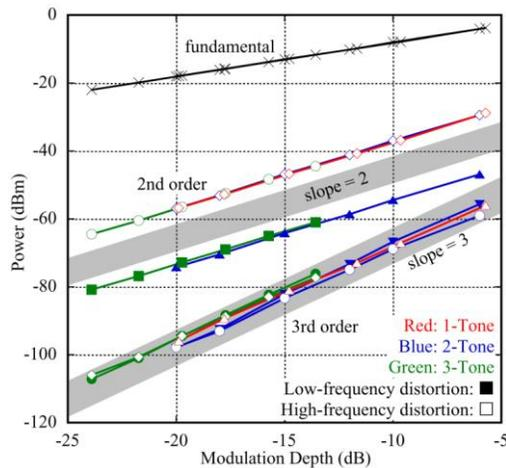
Fig. 7. Fundamental and selected second and third order distortion power versus modulation depth at 2.5V bias for a PD3000 photodiode. Fundamental frequency  $f = 100\text{MHz}$ , with frequency spacing  $\Delta f = 10\text{MHz}$  and total photocurrent = 10mA. One- and three-tone data are according to Eq. (10) and Eq. (11) to mathematically match the two-tone data.
