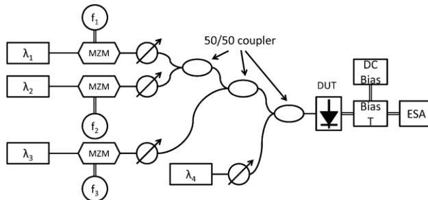
Fig. 2. Four laser three-tone MZM measurement setup
