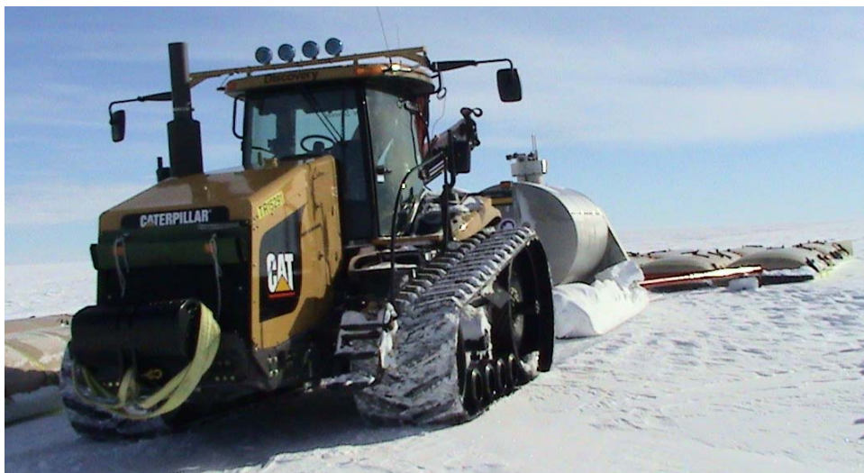
Figure 16. AGCO MT865 tractor with crane connected to a fuel tank and eight fuel bladders on HMW sleds for towing across a portion of the Ross Ice Shelf during SPoT 08-09.
