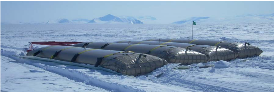
Figure 5. Four bladder sleds connected behind a spreader bar. Each sled consists of a 3000-gal. fuel bladder strapped to a flexible sheet of HMW-PE.
