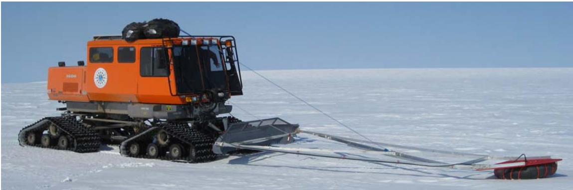
Figure 4. Tucker fitted with GPR antenna (inside inner tube) at the end of an aluminum boom.
