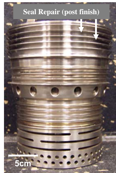
Figure 13. Inconel 718 Compressor Seal. Courtesy: RPM & Associates.
