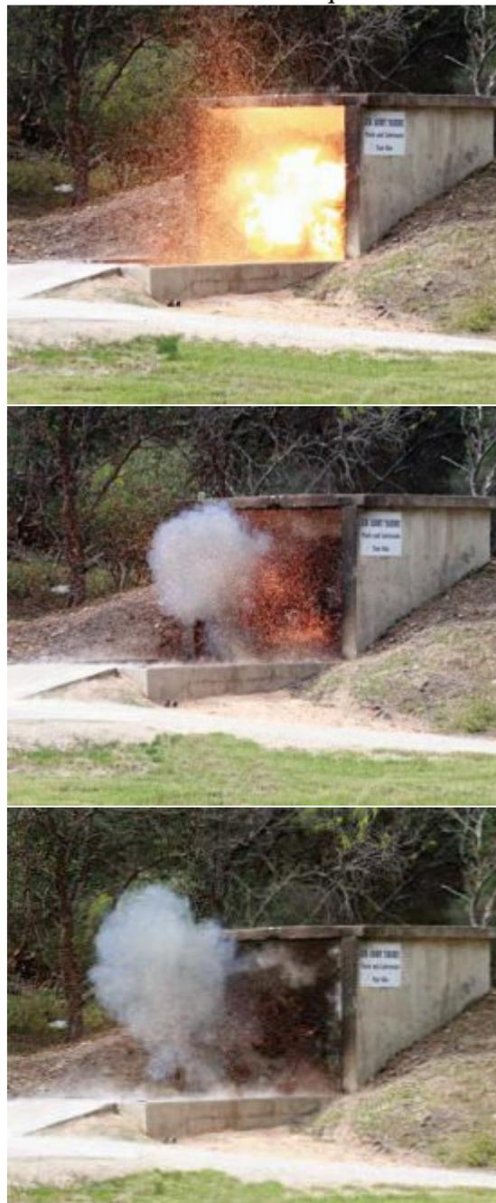
(U) Figure 1. Conventional JP8 compared to Diesel FRF
