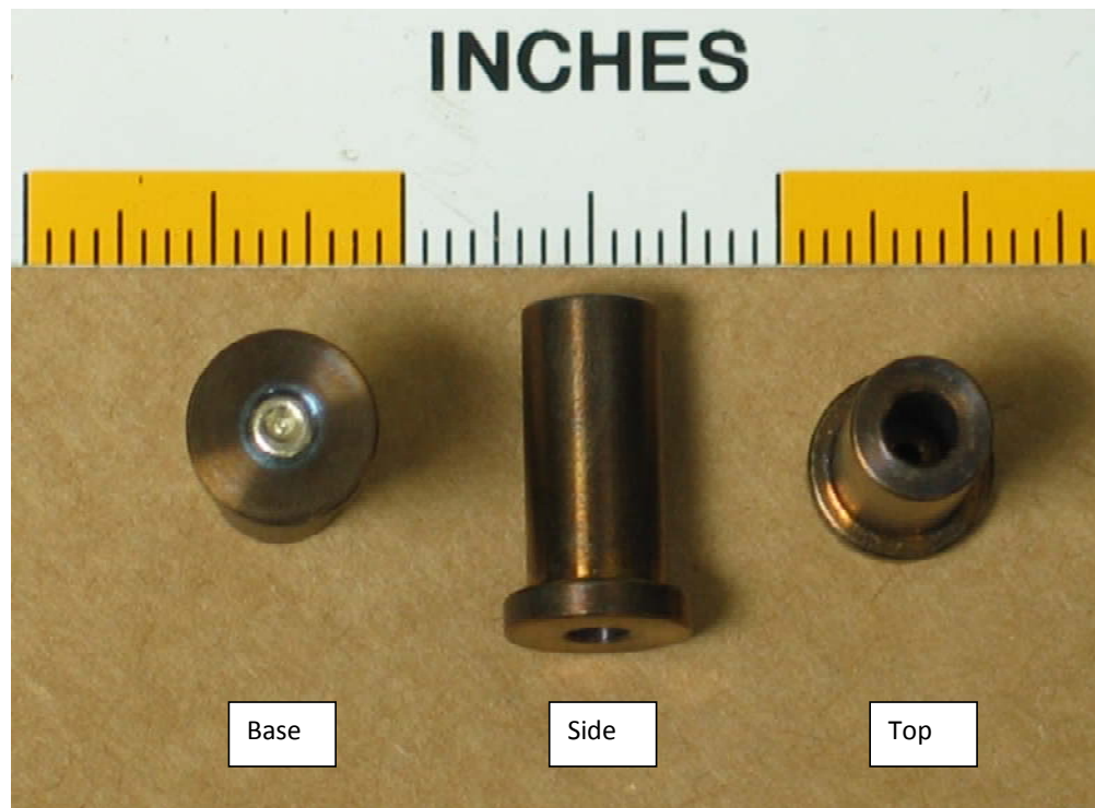
Figure 4. Photographs of the 0.22-cal. custom case.
