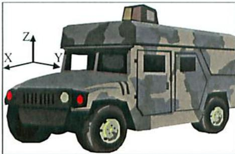
Fig. 4, Vehicle coordinate system
