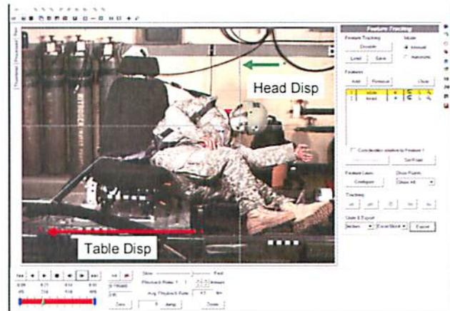
Fig. 5, Peak relative head excursion measurement
