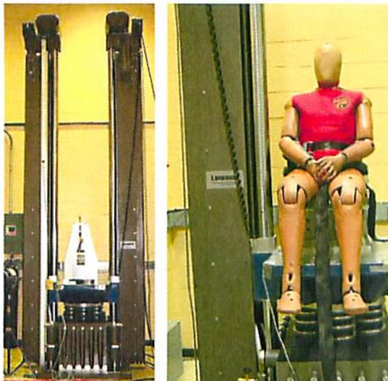
Fig. 2, Lansmont vertical shock machine (left), ATD seated on shock machine (right)
