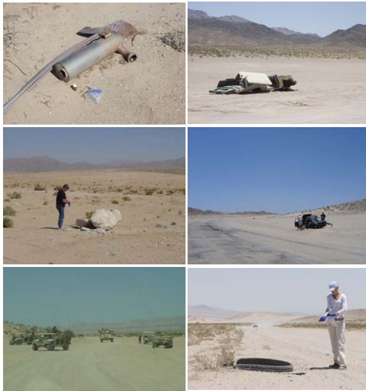
Figure 4. Objects and/or locations comprising “negative” threat truth where no known recent live-fire activity had taken place. Clockwise from upper right, military vehicle wreckage, civilian vehicle wreckage, a tire retread, a simulated VBIED event that did not use any live detonations, a suspicious roadside rock, and an abandoned vehicle muffler.
