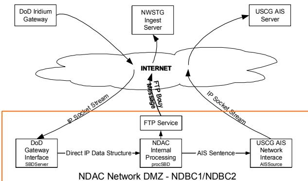
Figure 2. Shore-side Data Processing Flow
