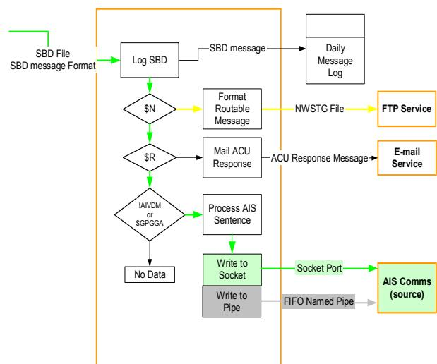
Figure 3. Short Burst Data Packet Processing
