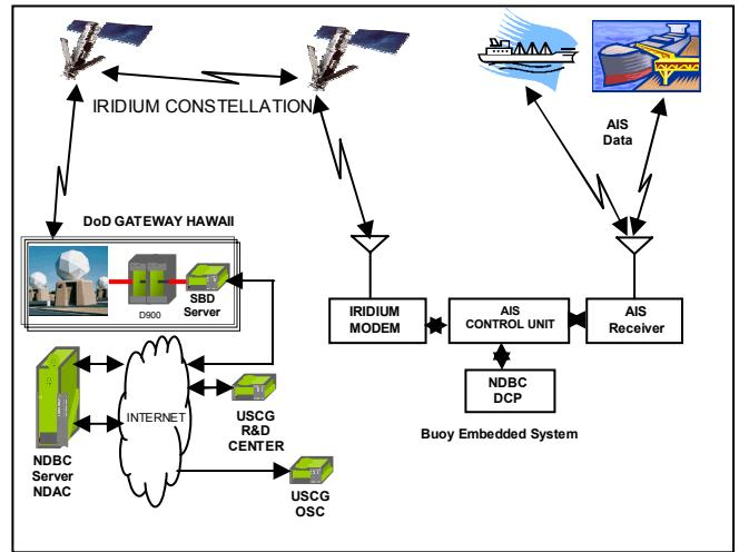
Figure 1. Block Diagram of Buoy AIS system
