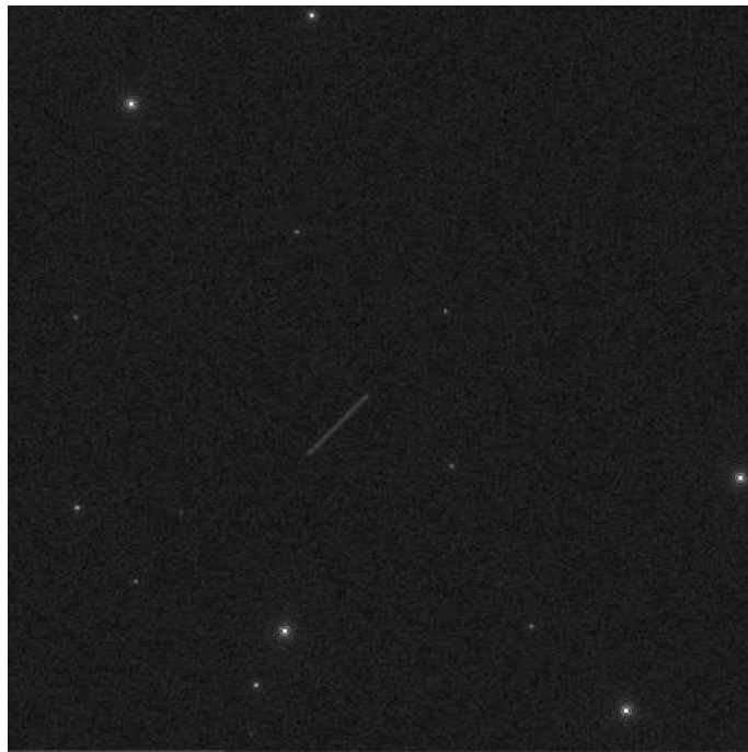
Figure 8. J-MAPS SSA Observation. RSO shown as a streak. RSO position is determined by measuring relative positions of streak endpoints with respect to reference stars of known positions.
