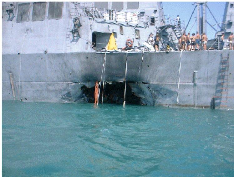
Figure 1. Damage to USS Cole Following Small Boat Attack<sup>32</sup>
