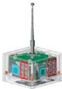
Figure 13. Inner processor and detectors of MSP410 mote (From xbow.com, September 2008)
