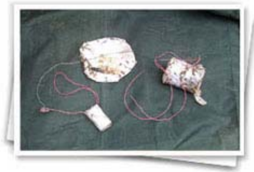
Figure 4. IED pressure switch (From eastarmy.nic.in, September 2008)
