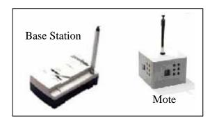
Figure 1. Crossbow MSP410 Base Station and Mote.
