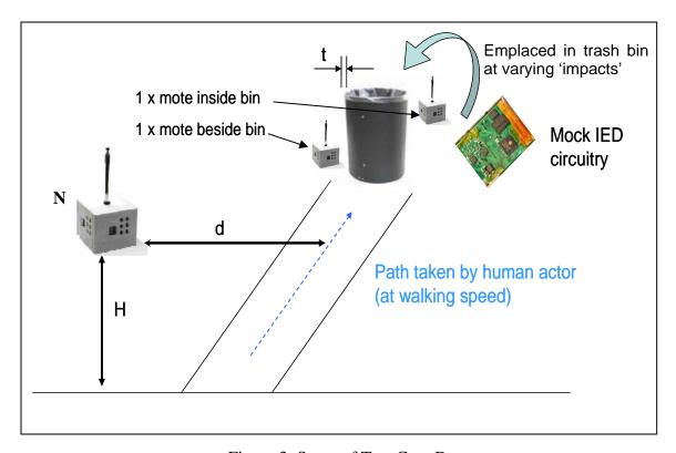
Figure 3: Setup of Test Case D.
