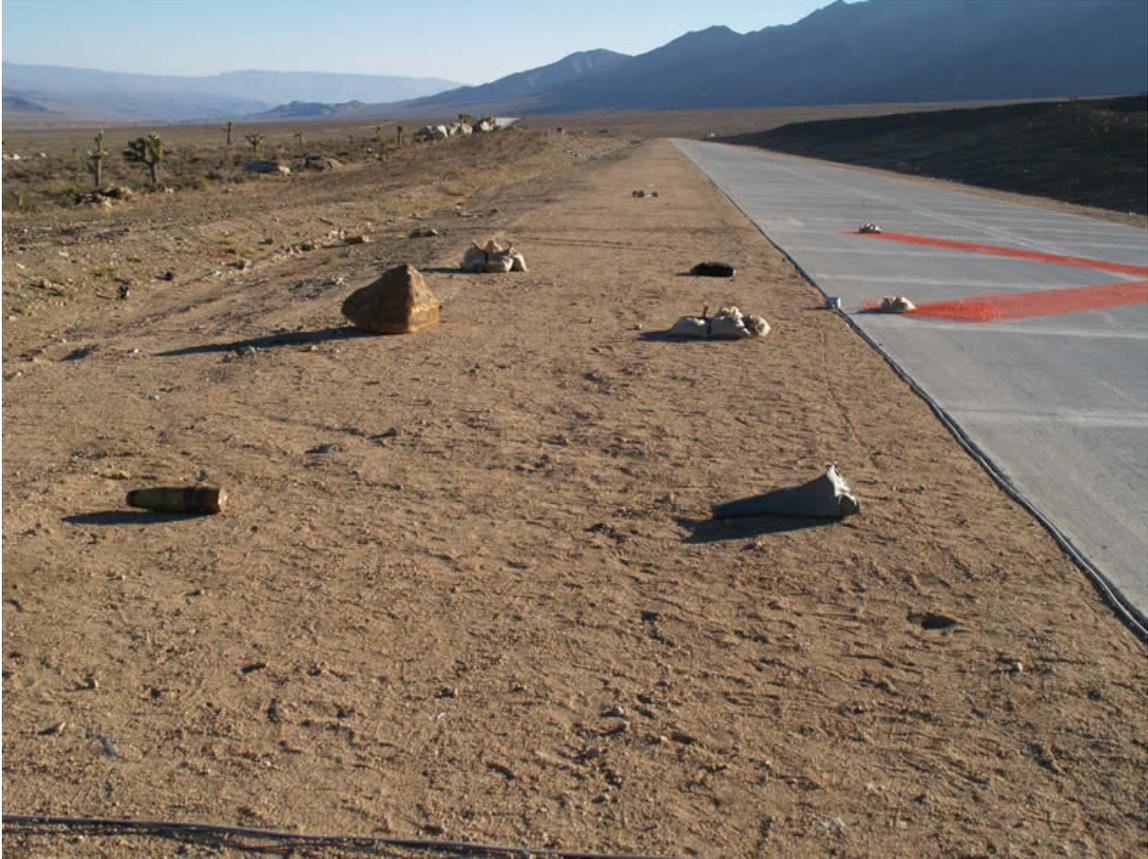
Figure 5. Photograph of targets in same orientation as the Figure 4 schematic. The triggering devices are in the ditch to the left and are almost impossible to detect on this photograph, as are the connecting wires. The red material on the runway forms a cross to aid the pilots in identifying the target location area.
