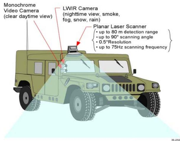
Figure 1. Video and LWIR cameras potential mounting positions.
