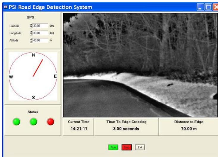
Figure 8. Conceptual design of the information shown to the driver
