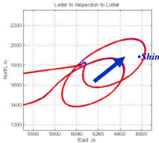
Figure 12, Simulated Target Ship Inspection Track Generation and Following.
