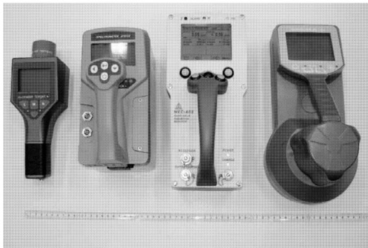
Figure 3. Hand-held radiation detectors and survey instruments (From: *Combating Illicit Trafficking in Nuclear and other Radioactive Material*, 2007, p. 108)
