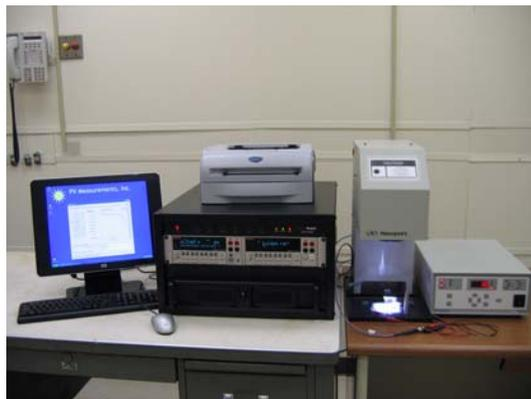
Figure 6. The new ARL solar cell I-V curve testing system.
