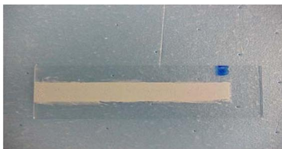
Figure 3. An example of a coating of  $\text{TiO}_2$  on conductive (F-doped  $\text{SnO}_2$ -coated) glass.
