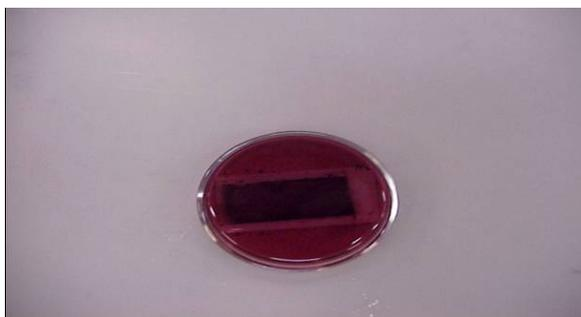
Figure 4. TiO<sub>2</sub> film adsorbing the solar dye.
