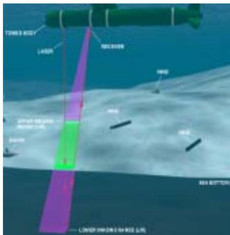
**Figure 1. EOID Scanning Scheme for Target Identification**
