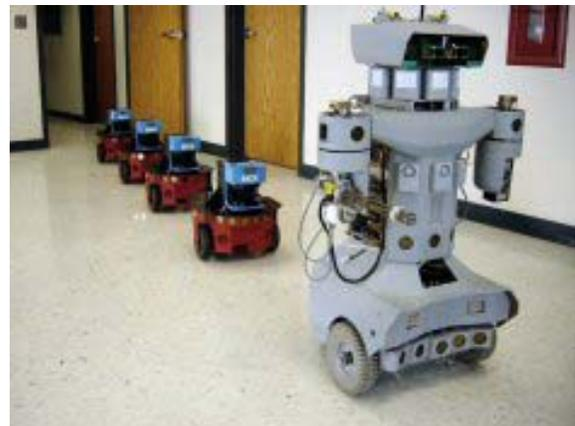
**Figure 1.** Convoy formation with SSC-SD's Robart III as the lead robot followed by Pioneer 2DX relay robots.
