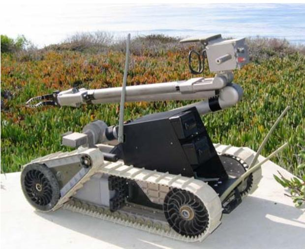
**Figure 4.** Deployer module with two Relay Bricks, mounted on the EOD PackBot.
