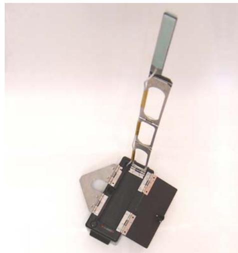
**Figure 2.** Relay Brick, open with antenna mast extended.
