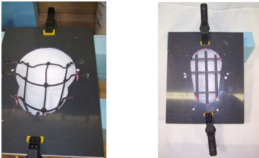
Figure 3. Mask form holder constructed from PVC
