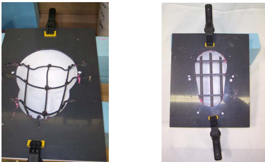
Figure 3. Mask form holder constructed from PVC
