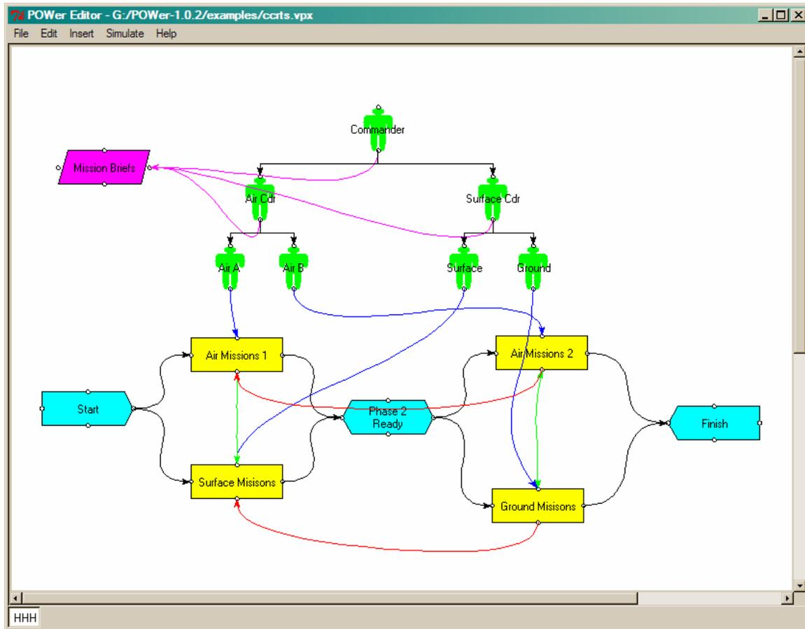
**Figure 2 POW-ER Model Editor.** A graphical model editor is the primary means of entering models into POW-ER. Shown above is a simple command and control (C2) model, which is described in the article (Nissen and Buettner, 2004). The diagram represents actors, tasks, milestones, and meetings, along with the relationships between them.
