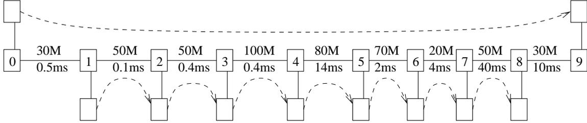
Figure 5: Testbed configuration. Hop 0 is the probing sender, hop 9 is the probing destination. Hop 1 - 8 work as routers, and we use  $R1 - R8$  to denote them in the paper. The blank boxes are used for background traffic generation. The dashed lines show the background traffic flow directions for the evaluations in “single bottleneck” and “two bottlenecks”.
