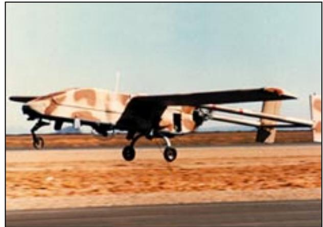
**Figure 6.** Pioneer RQ-2 unmanned aircraft.
