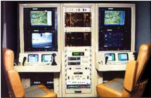
**Figure 11.** Predator ground control station layout.
