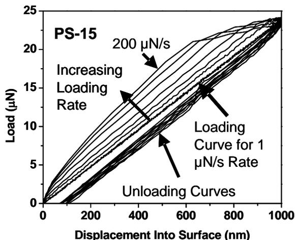
**Figure 5:** Loading and unloading curves for loading rates of (1, 10, 25, 50, 100, 150 and 200)  $\mu\text{N/s}$  on PS-15, illustrating the time-dependent response of the material. Results were similar for PS-30.
