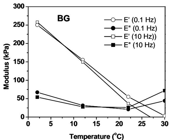
**Figure 2:** Storage and loss modulus properties for BG as measured dynamically at 0.1 and 10 Hz with the rheometer from 0-30 °C. Properties vary greatly as a function of temperature.
