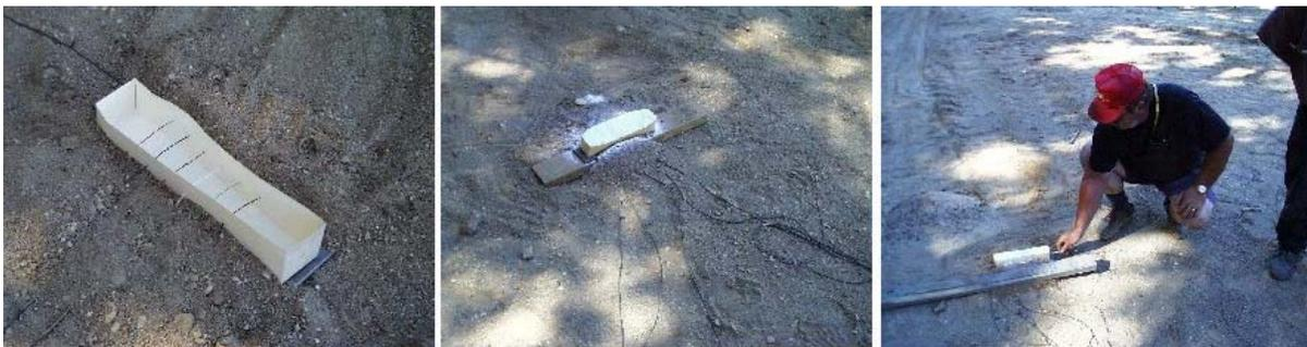
Figure 1 Experimental set-up for measuring Detonation velocity of LEXFOAM in a paper tray at 88<sup>0</sup>F
