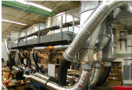
Figure 8. High-speed, high accuracy evaluation of full scale HVAC/air cleaning equipment at the NREL Advanced HVAC Laboratory
