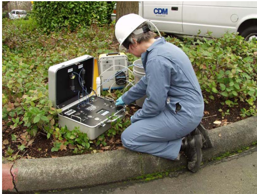
Figure 2. Dissolved Hydrogen Analyzer Implementation.
