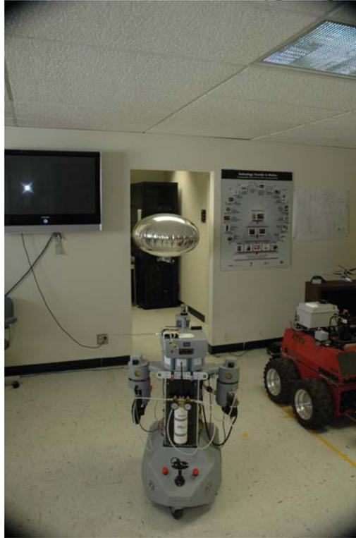
**Figure 11** ROBART III teleoperating a 3-foot diameter Mylar aerostat
