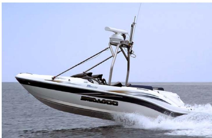
Figure 1. SSC San Diego USV operating autonomously in open water
