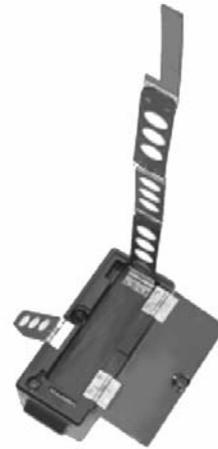
**Figure 5.** The prototype Relay Brick automatically self-rights and deploys its antenna.
