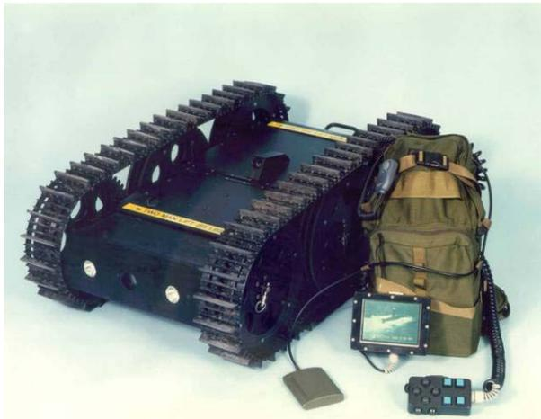
**Figure 1.** The MPRS URBOT and its backpack controller.
