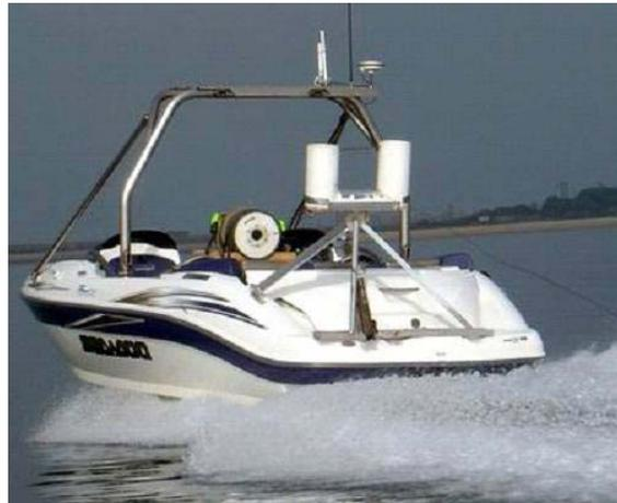
**Figure 2.** The USV demonstrating autonomous deployment of fiber-optic cable.
