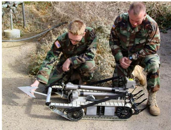
**Figure 9.** The iRobot Tool/Lift Kit. The universal tool mount is on the left (front of the robot).
