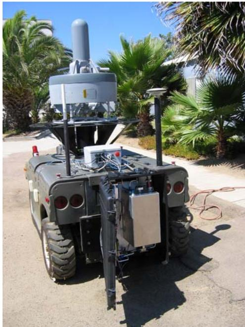
**Figure 6.** The AUMS configuration with the MDARS UGV and *iSTAR* UAV. The refueling system can be seen attached to the back of the UGV.
