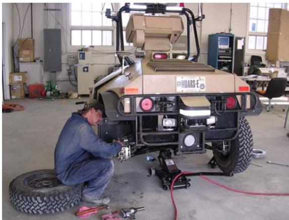
Figure12. MDARS Trained Mechanic Working On The Brakes
