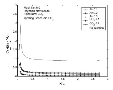
Fig 1. variation of skin friction for injection of different gases for M=6.0 and R=10.6
