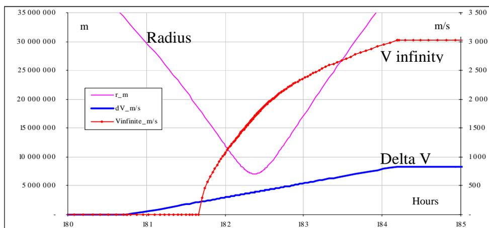
**Figure 9 Delta V to be provided by the low thrust propulsion to reach the Mars orbit transfer from a high elliptic Earth orbit.** The velocity infinity (escape velocity) of the hyperbolic branch starts to be positive around the lowest radius (perigee), the location of highest efficiency to increase the V infinity.
