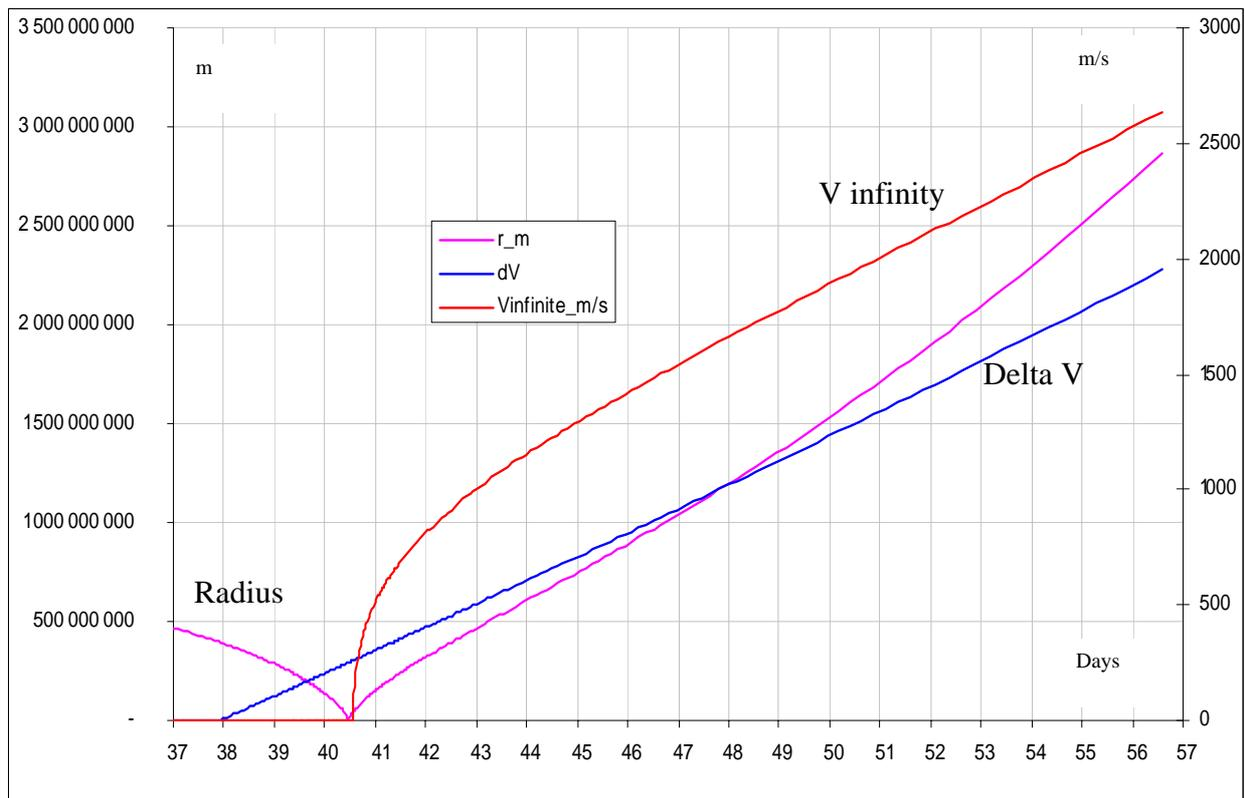
**Figure 7** *Delta V to be provided by the low thrust propulsion to reach the Mars orbit transfer from a high elliptic Earth orbit.* The velocity infinity (escape velocity) of the hyperbolic branch starts to be positive just at the lowest radius (perigee), the location of highest efficiency to increase the V infinity.
