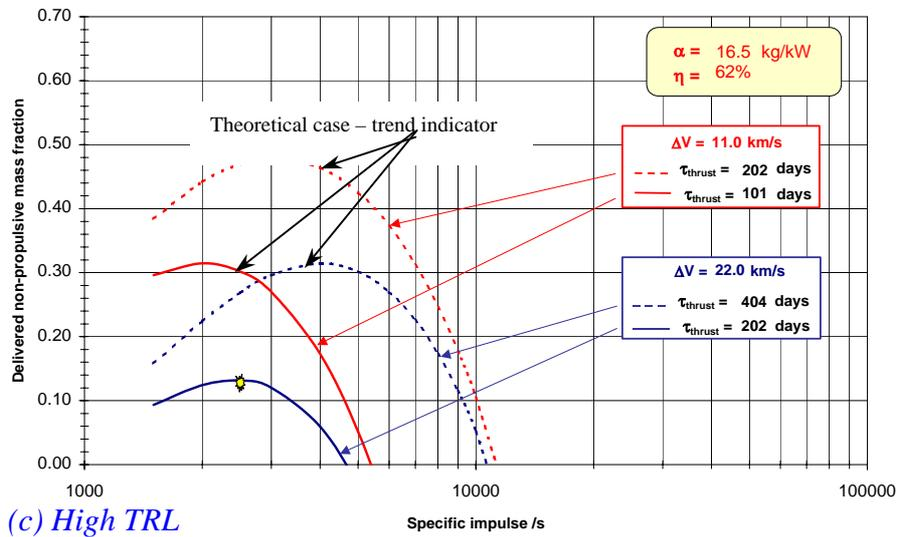
**Figure 3** *Delivered mass fraction as a function of  $I_{sp}$  for two values of  $\Delta V$  and acceleration.* Figures a (top) through c (bottom) illustrate the effect of increasing the TRL indeed, increasing the system  $\alpha$  (kg/kW) on mission performance and optimum  $I_{sp}$ . For short thrust duration (101 days), the optimum  $I_{sp}$  is in the range 1500 to 2500 s for values of  $\alpha = 16.5$  kg/kWe.
