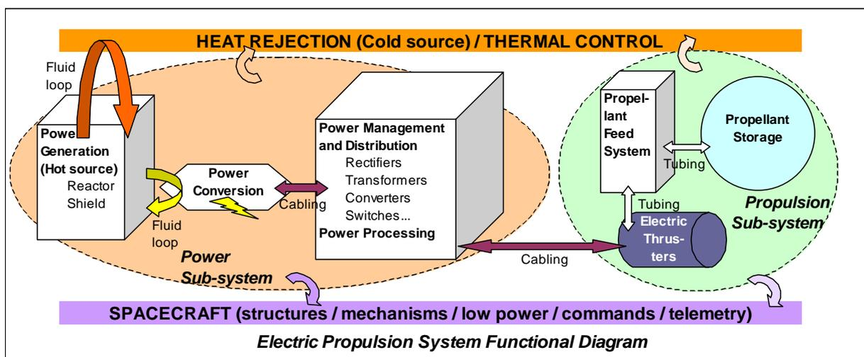
**Figure 2** *Nuclear electric propulsion system schematic diagram*
