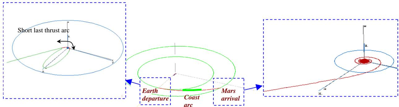
**Figure 8 Mission from LEO to LMO with Electric propulsion and higher thrust chemical propulsion.** The electric propulsion is used along arcs at departure followed by a short arc of higher chemical thrust, and electric propulsion is used continuously at arrival.
