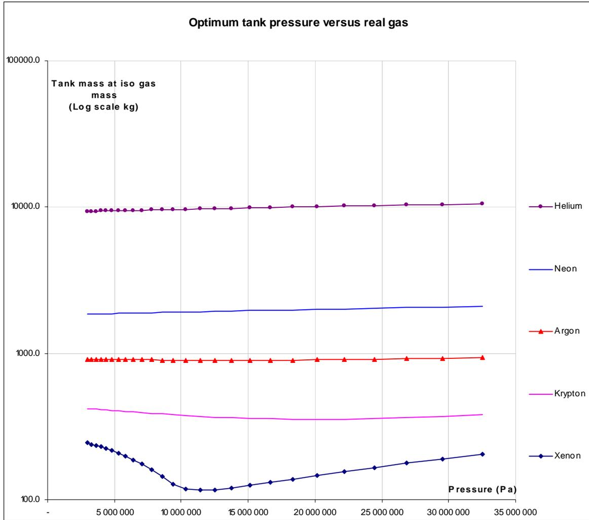
**Figure 4** Optimum gas pressure for various gases in composite tanks. The xenon presents a real optimum around 15MPa, krypton optimum is quite flat, while for the other gas the minimum pressure is recommended when considering only the mass criteria.
