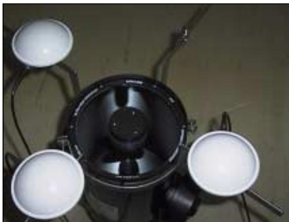
GPS antennas mounted on the telescope (front view)
