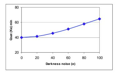
**Figure 2.** Minimum charge storage capacity requested as a function of darkness noise.
