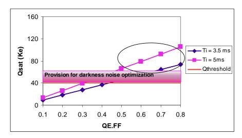
**Figure 4**. Relationship between Qsat and QE.FF, assuming H=700 km; D=0.3 m; KTel=0.7;  $\Delta\lambda$ =0.25 $\mu$ m;  $\lambda$ =590 nm.
