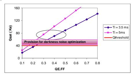
**Figure 3**. Example of relationship between Qsat and QE.FF, assuming H=600 km; D=0.3 m; KTel=0.7;  $\Delta\lambda$ =0.35 $\mu$ m;  $\lambda$ =650 nm.
