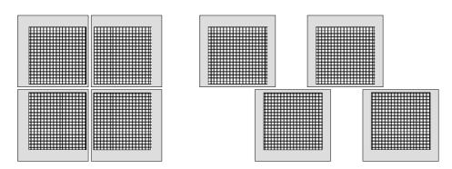
**Figure 1**: 8kx8K focal plane architecture with 4 butted devices and 16Kx8K focal plane architecture with 4 staggered devices.
