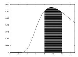
Figure 2: The Planck curve for a black-body at 303K (roughly skin temperature), with the area to be integrated for an  $8-12\mu m$  sensor shaded.
